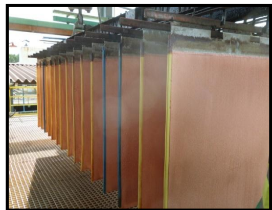
Figure 16 Extracted copper plate from Tank House
